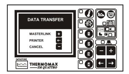
(c) To download data to the Masterlink Hardware unit, (Part No. C0321), press the key and the following screen will appear:
