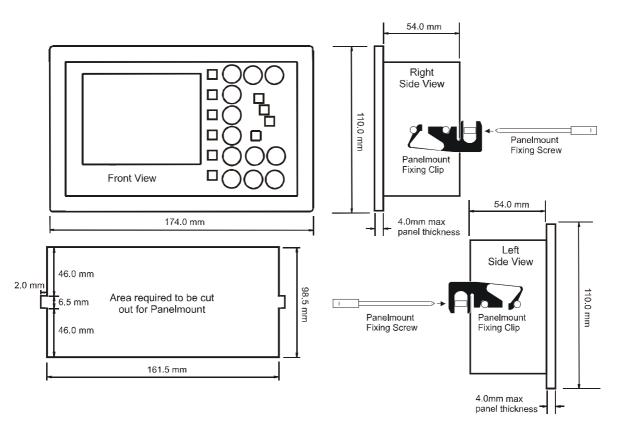
After inserting the Panelmount unit into the panel cut out, attach the two panelmount fixing clips (supplied), to the two studs at either side of the unit, (as above). The Panelmount unit is then held in place by the two Panelmount fixing screws (also supplied).
