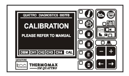
To enter the CALIBRATION TRIMMING Screen, press and hold the for 5 seconds.
