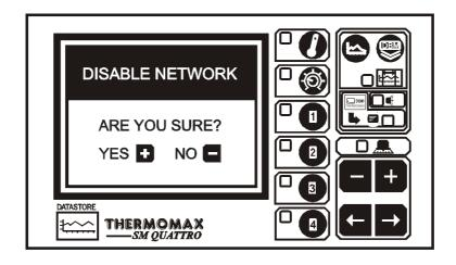
To disable the network press the key. (When the key is pressed, the SM Quattro will switch off and back on again).
