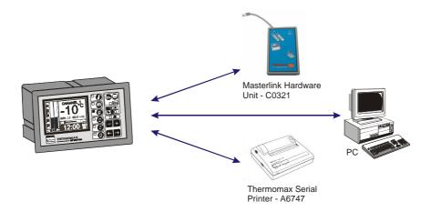
Mode 2 This mode is used to network up to 32 units to one PC, (see illustration below).
