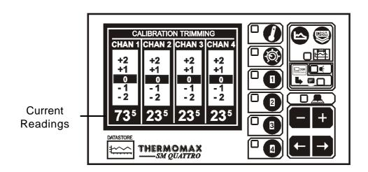
Use the keys to move to the channel which requires calibration trimming. Then use the or keys to adjust the current temperature reading.
