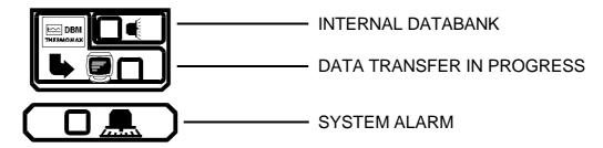
The System Alarm can be triggered by the high temperature alarm, low temperature alarm, or by a sensor fault.
