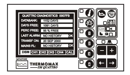
With this screen displayed, press and hold the key for approximately 10 seconds. The following screen will appear:
