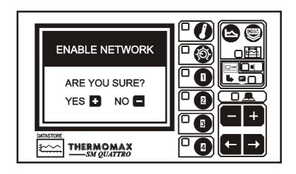
To enable the network press the key. (When the key is pressed, the SM Quattro will switch off and back on again).
