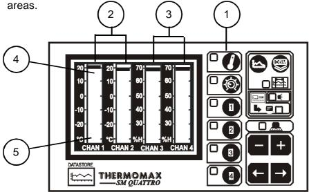
Pressing the key the first time will display the MAIN SCREEN which shows a four channel bargraph display as shown above.
